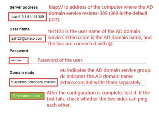
PS: The following uses 1 | Idap://192.168.213.196:389, Username: test111@test.com, Domain node: ou=pers,dc=test,dc=comas an example
