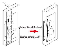
Align the template along the vertical center line of the latch(D) at the desired handle height, and tape it to the door.
