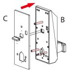
3.2 Insert spindle(H) into the clutch.
