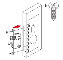
**Note:** Installing the mortise(D) on the door by inserting screws(E).
