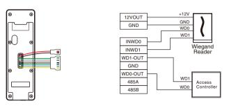
**Note:** 485A and 485B can be connected to the Barrier gate or the 485 Reader, separately, but cannot be connected to the gate and reader at the same time.
