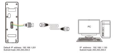
Click on [COMM.] > [Ethernet] > [IP Address], input the IP address and click on [OK].
