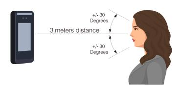
While most of algorithms only support 15-degree angle facial recognition, Armatura supports 30-degree angle facial recognition.
