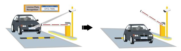
LPR Camera scan the number on the license plate when vehicle is approaching its reading range.
