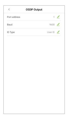
• The device can connect the external devices such as a printer via RS232, OSDP output is used for setting the Serial port address, Baud rate and ID type.
