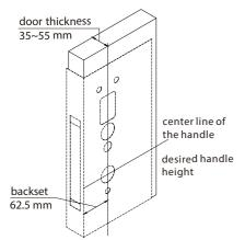
Note 1: Align the template along the vertical center line of the mortise (G) at the desired handle height, and tape it to door. Note 2: Mark the holes first, then start drilling.
