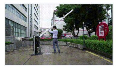
If the boom arm can move up smoothly to the desired position, it indicates that both the mechanical moving part and the motor movement are functioning properly.
