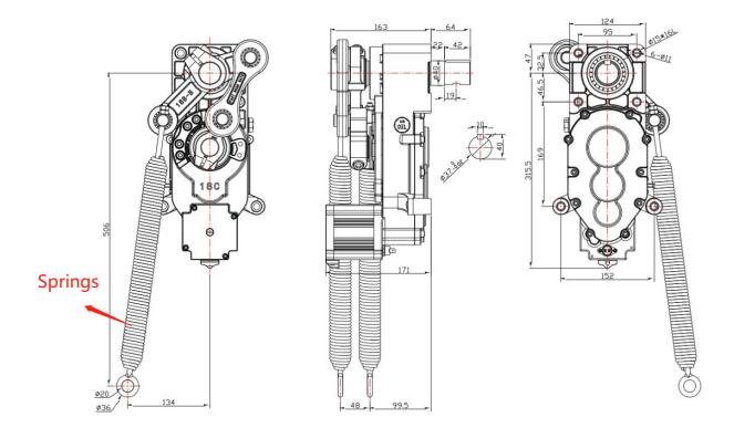
The spring is used to balance the weight of the boom arm when it moves down to the horizontal position. The quantity of springs required depends on the length and diameter of the boom arm.
