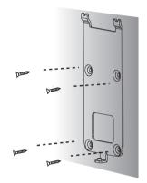
(4) Fix the back plate on the wall according to the mounting paper.
