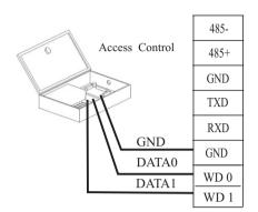
The device has the function of Wiegand signal input. It supports to connect with an independent card reader. They are installed each side of the door, to control the lock and access together.
