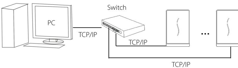
The default IP address is 192.168.1.201. IP addresses of the server (PC) and the device must be in the same network segment.
