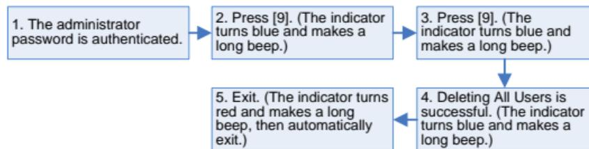
😊**Note:** In step 3, press [9] for automatic confirmation. Other numbers are considered invalid. If an invalid number is entered, the device indicator turns red, and the device makes a long beep and exits the process.
