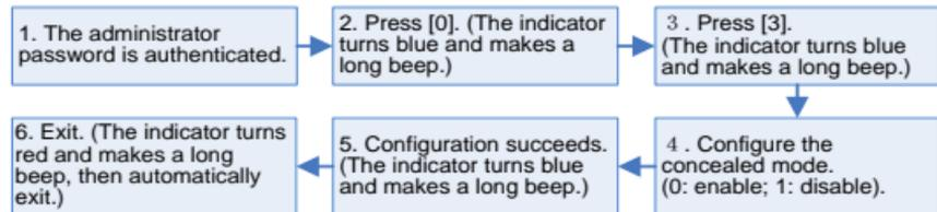
😊**Note:** When user is authenticating the card or password under Concealed Mode, the indicator will still blink correspondingly to denote process status.
