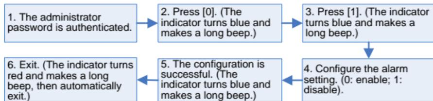
**Note:** The Tamper Alarm is still effective even if the alarm switch is OFF.
