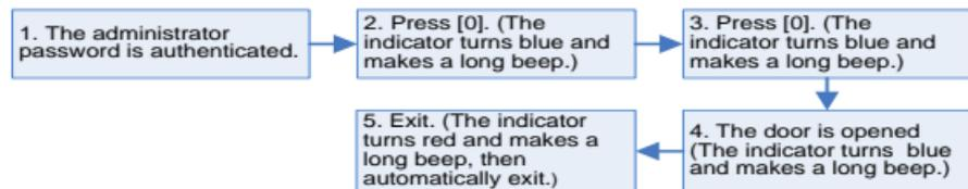
😊**Note:** This function can be used to open the door.
