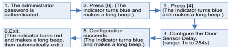
☺**Note:** Three-digit values will be automatically verified. For values with less than three digits, press [#] to confirm. Values greater than 254 are considered invalid.
