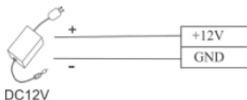
Input DC12V,  $\leq 110mA$  ( $\leq 80mA$  standby) Positive is connected with **+12V**, negative is connected with **GND** (do not reverse the polarities).
