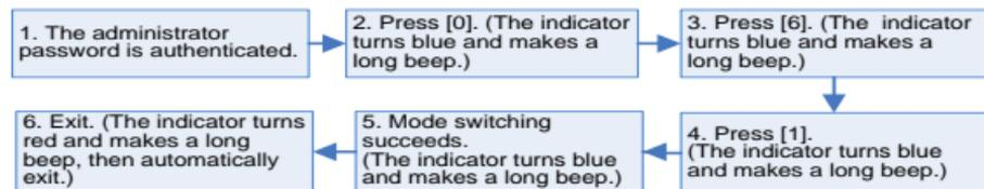
😊**Note:** When mode switching fails, the device will give 3 short beeps, followed by the indicator turning to red with a long beep, and then automatically exits.
