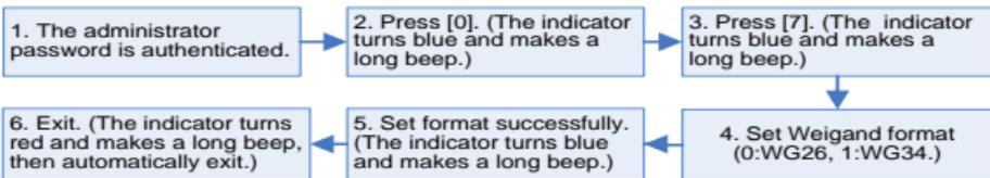
😊**Note:** When mode switching fails, the device will give 3 short beeps, followed by the indicator turning to red with a long beep, and then automatically exits.
