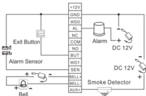
Only devices with an alarm  $\leq DC 12V$  can be connected.
