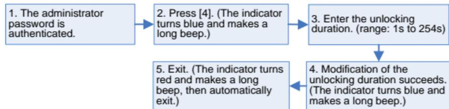
😊**Note:** The unit of unlocking duration is “second”. Three-digit values will be automatically verified. For values with less than three digits, press [#] to enter verification process.
