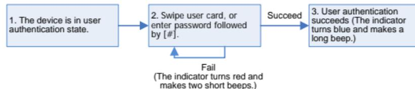
😊**Note:** Press [#] after entering a password for authentication. The door opens if the entered password is identical passwords for opening the door.
