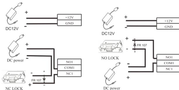
(1) The system supports NO LOCK and NC LOCK. The NO LOCK (normally open by power on) is connected with NO terminal, and the NC LOCK is connected with NC terminal.
