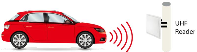
Note: To get better reading performance, driving direction of vehicle should face to the UHF integrated machine.
