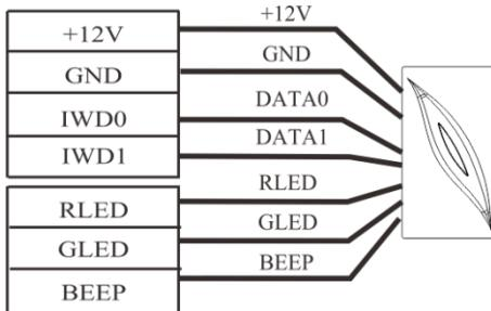
The device has the function of Wiegand signal input. It supports to connect with an independent card reader. They are installed each side of the door, to control the lock and access together.
