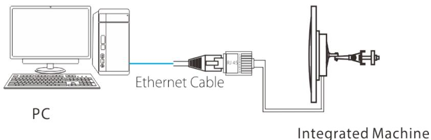
Connect the RJ45 port of the integrated machine to the Ethernet port of the computer. The machine supports access to ZKAccess 3.5 and ZKBioSecurity 3.0.
