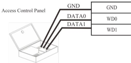
The device supports standard Wiegand 26/34 output, as a reader device it has a very good compatibility.
