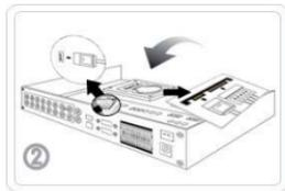
② Install the HDD into the HDD bracket and connect the HDD cable
