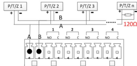
**Note:** 120Ω resistors should be paralleled in the remote A, B lines to reduce the distortion of the signal if a larger number of PTZs are connected.
