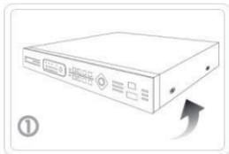
① Remove the screws of the device and disassemble the cover
