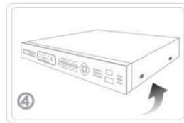
④ Close the cover and assemble the screws to fix the cover
