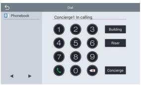
Click " concerned" icon to call master station, the system will call master station No.1-No.5 successively. If the master station cannot be searched or call failed, the system will automatically call next master station. When the master station answers, it will ring and stop calling next one.
