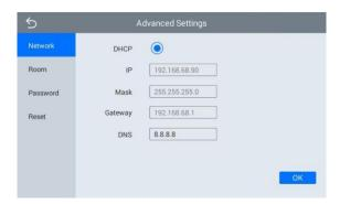
After using the DHCP, the router will automatically distribute IP address. Other settings are the same as the ones of Smart Life APP. IP: Static IP address.
