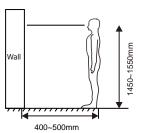
[Suggestion]: During the installation, the camera should be  $1450 \sim 1550 \text{mm}$  above the ground. The camera tether for photographing human face should be the top priorit
