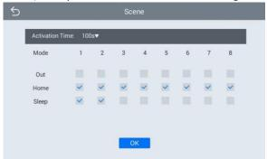
refers to Alarm ON, refers to Alarm OFF. To set the sensor of alarm stations, you can click the corresponding station with icon. Click "Activation Time" to select the corresponding time. The options of activation time include NONE, 30s, 40s, 60s, 100s and 300s.
